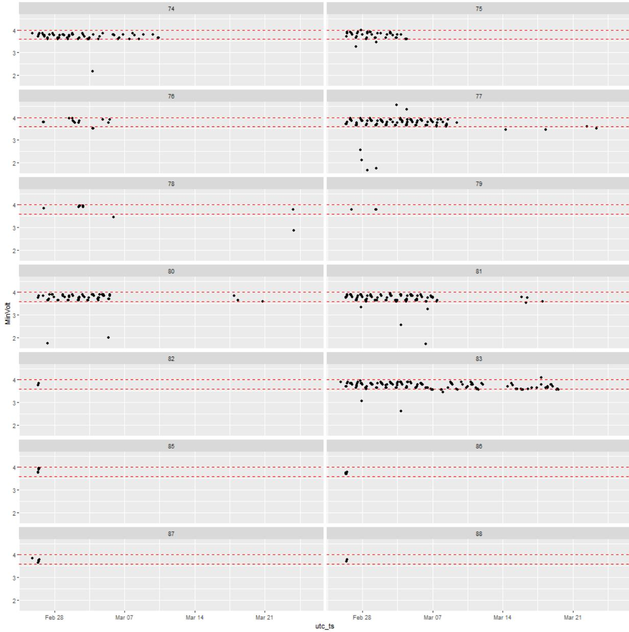
**Figure 3. Plots of tag battery voltage (V) values over time for all data collected following tag deployment. Red dashed lines show values in healthy range.**
