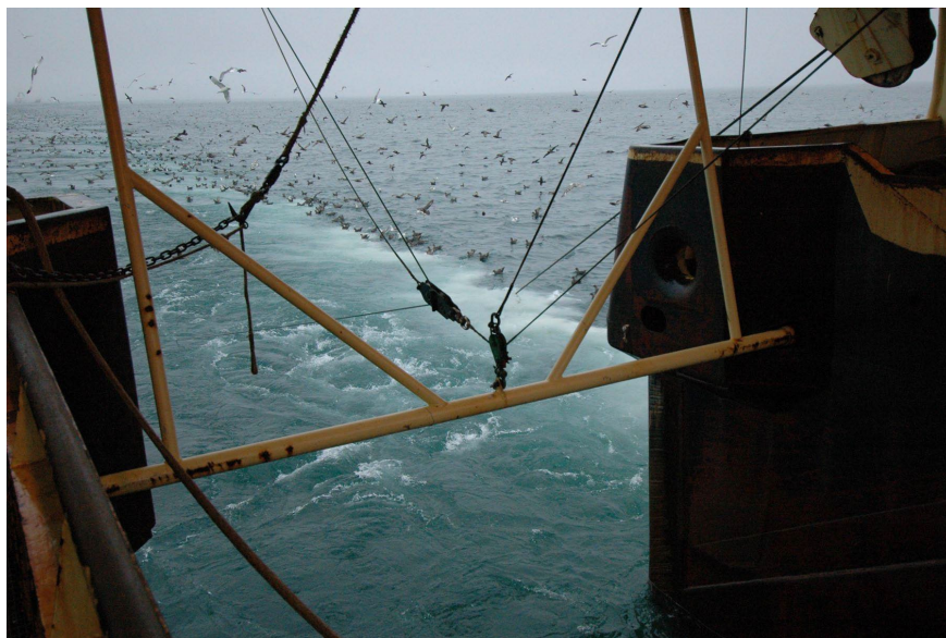
Figure 1. Example of a snatch block (i.e., pulley in the center of the image that is directing the angle of the cables). Photo credit: Ed Melvin
