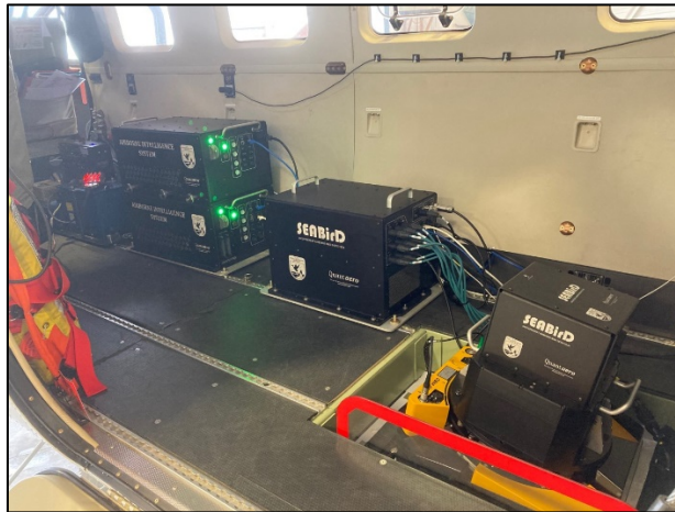
Figure 1. High-resolution camera array integrated with direct geo-referencing system and in-flight data processing components mounted in U.S. Fish and Wildlife Service aircraft.
